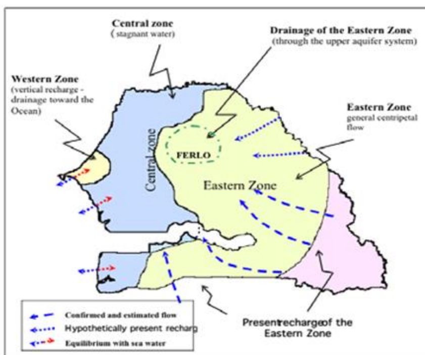
Figure 1: Conceptual flow model of the Maastrichtian Aquifer System in Senegal 1
